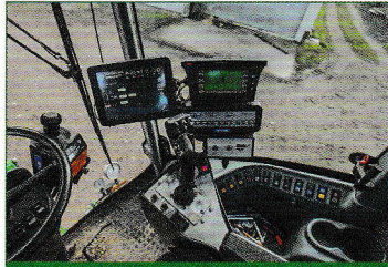
Up in the cab, Paul uses Trimble EZ-Steer and EZ-Boom to make the most of GPS.
