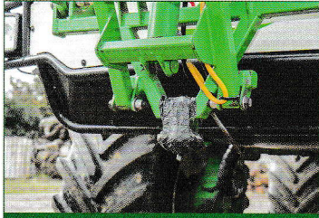
Paul wraps duct tape over this bracket to prevent it from snagging on tall crops.
